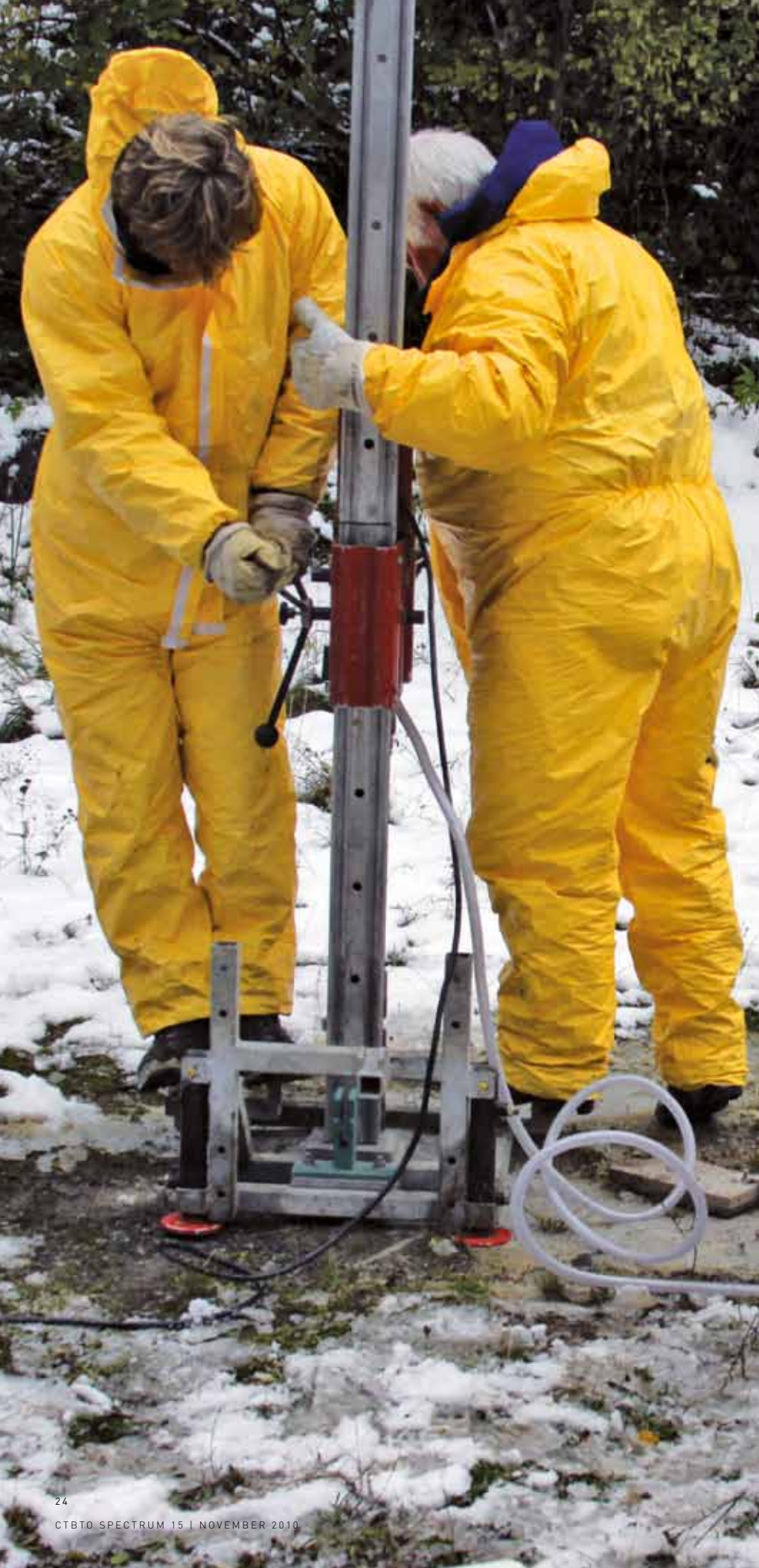
Augering a shallow hole as a preliminary to setting up a noble gas sampling site during NG09.
