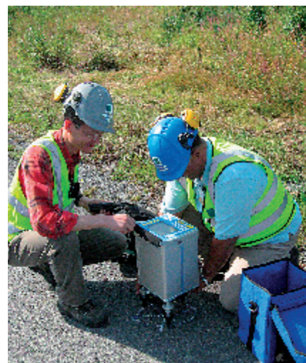
Relative gravimetric measurement during the directed exercise, Finland, July-August 2009.
