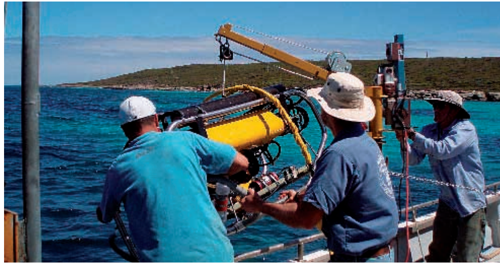
Hoisting a remotely operated vehicle into the water to take video recordings of the data transmission cable connecting the hydrophones of hydroacoustic station HA1 to the shore at Cape Leeuwin, Western Australia, during inspection in 2009.
