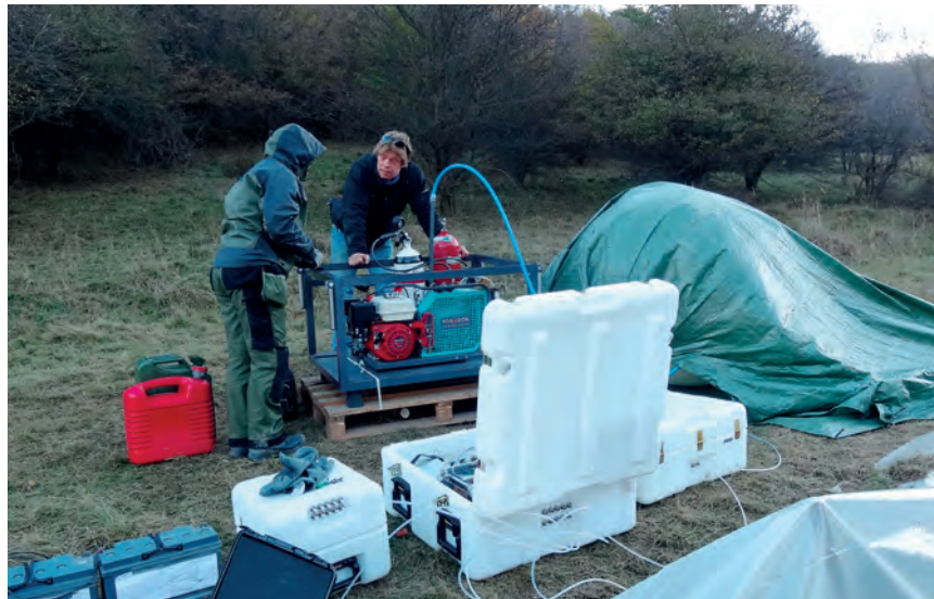
Testing of a smart sampler developed for OSI purposes (as a contribution in kind by the USA) during a field test of noble gas subsoil sampling techniques, Slovakia, October 2012.
