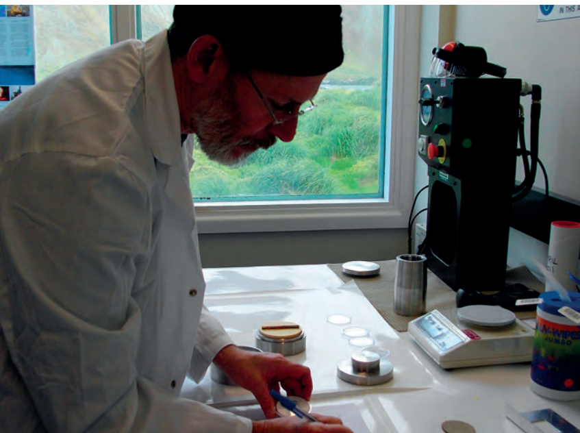
Radionuclide station RN7, Macquarie Island, Australia, which was certified in 2012. Left: Preparation of filter after removal from air sampler (right).
