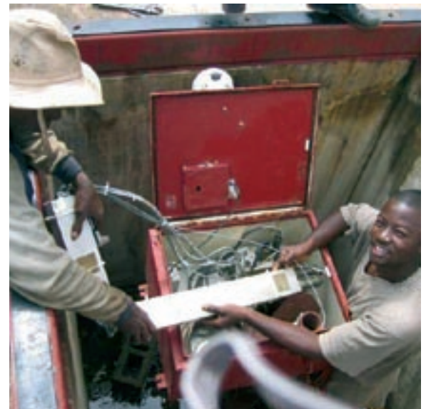
STATION OPERATOR WORKING ON WELLHEAD ELECTRONICS AT SEISMIC BOREHOLE, PS15, DIMBOKRO, COTE D'IVOIRE
