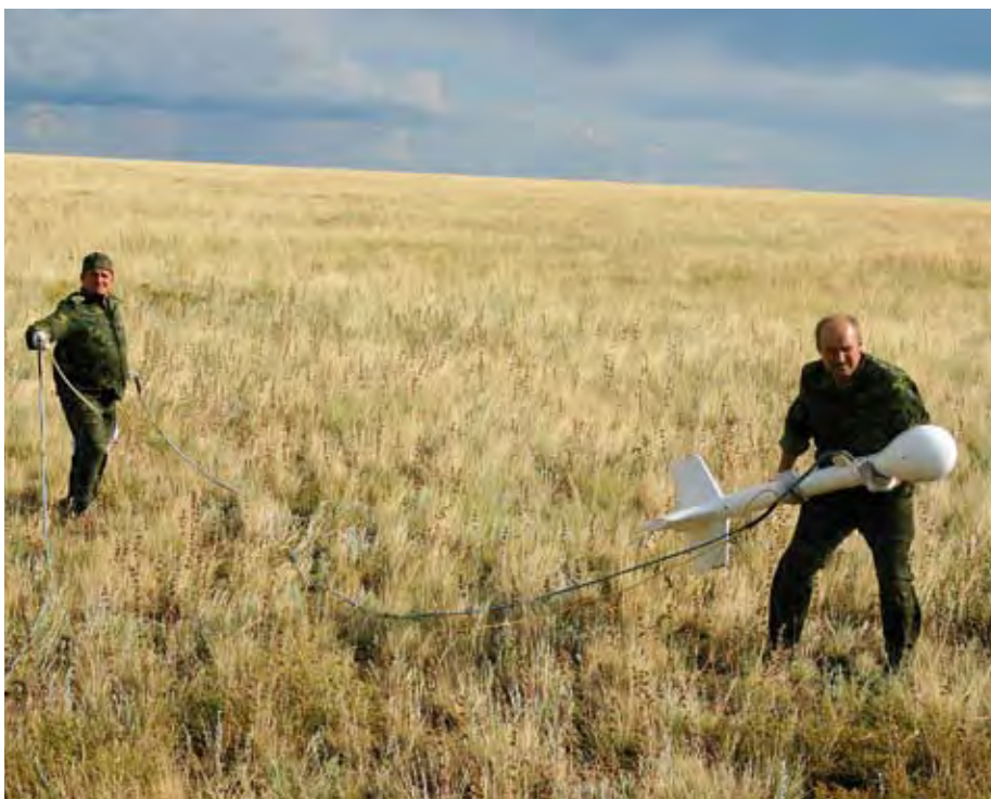
PREPARING TO FLY A MAGNETIC PROBE. THIS IS ONE OF THE OSI TECHNIQUES THAT WAS EXERCISED IN THE KAZAKH STEPPE IN 2005.
