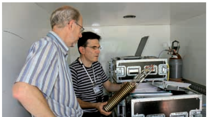
The charcoal column of the mobile SAUNA system installed in a truck. Concentrated radionuclide was collected in the column during the field measurement campaign in Belgium, which was jointly sponsored by the Swedish Defence Research Agency.
