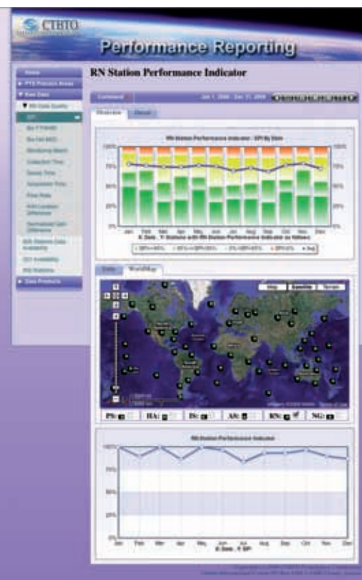
Example of KPIs displayed using the prototype performance reporting tool. The upper chart shows the station performance indicator for the IMS radionuclide monitoring technology during 2008. The lower graph shows the performance indicator for one of the stations shown on the map.
