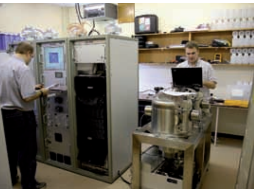
SAUNA-II equipment provided by the Pacific Northwest National Laboratory, Richland, Washington, USA, at the North-West University in Mafikeng, South Africa, during its deployment in the third noble gas measurement campaign in November–December 2008.
